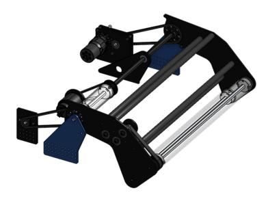
The intake allows for quick pickup and passoff of notes.
