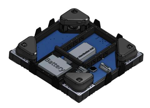
The Drivebase allows our robot to move across the field quickly and efficiently. We chose the swerve drive because it allows more maneuverability than the tank drive and has more defense resistance than the H-Drive or Mecanum.
